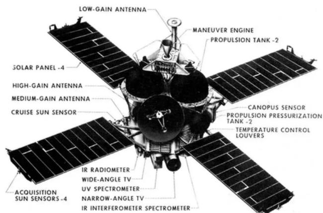
**Figure 6.** Mariner 9, based on the earlier spacecraft, but with larger propellant tanks to allow slowing and orbital capture at Mars. Credit: NASA/JPL-Caltech.
