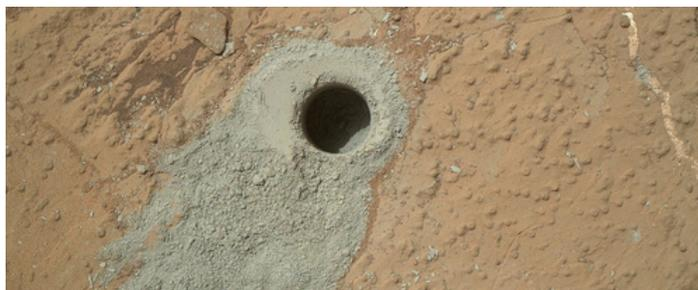
**Figure 12.** Curiosity's tools include a drill to obtain subsurface samples. Credit: NASA/JPL-Caltech/MSSS.
